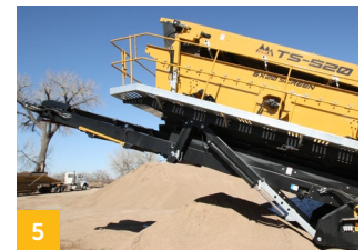
5 Hydraulic Screenbox linkage system, allows greater accessibility for screen change and enables optimum screen coverage at varying screenbox angles.
