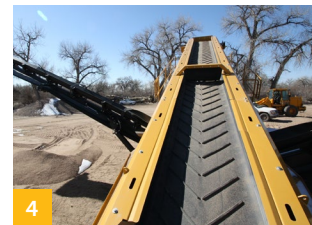
4 48" (1200 mm) feed conveyor enables high capacity screening.
