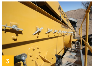
3 User friendly wedge system ensures faster screen changes.
